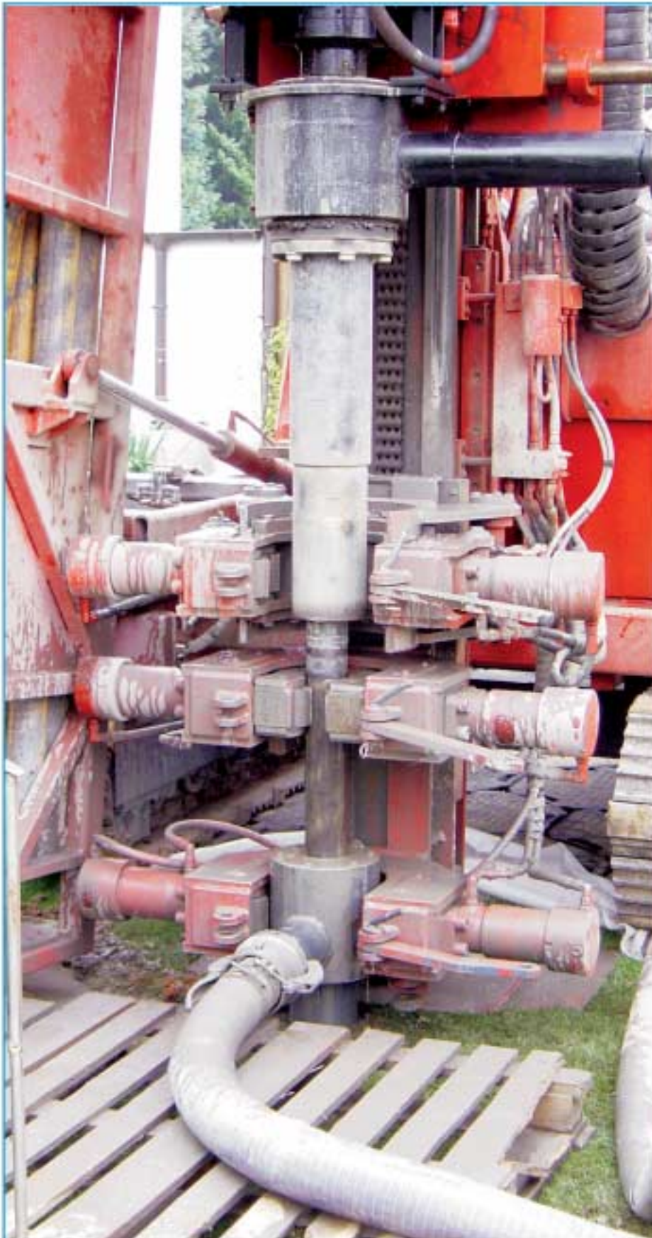
Upper and lower preventer on double rotary head type HG24/HG12. Three-fold clamping and breaking device.
