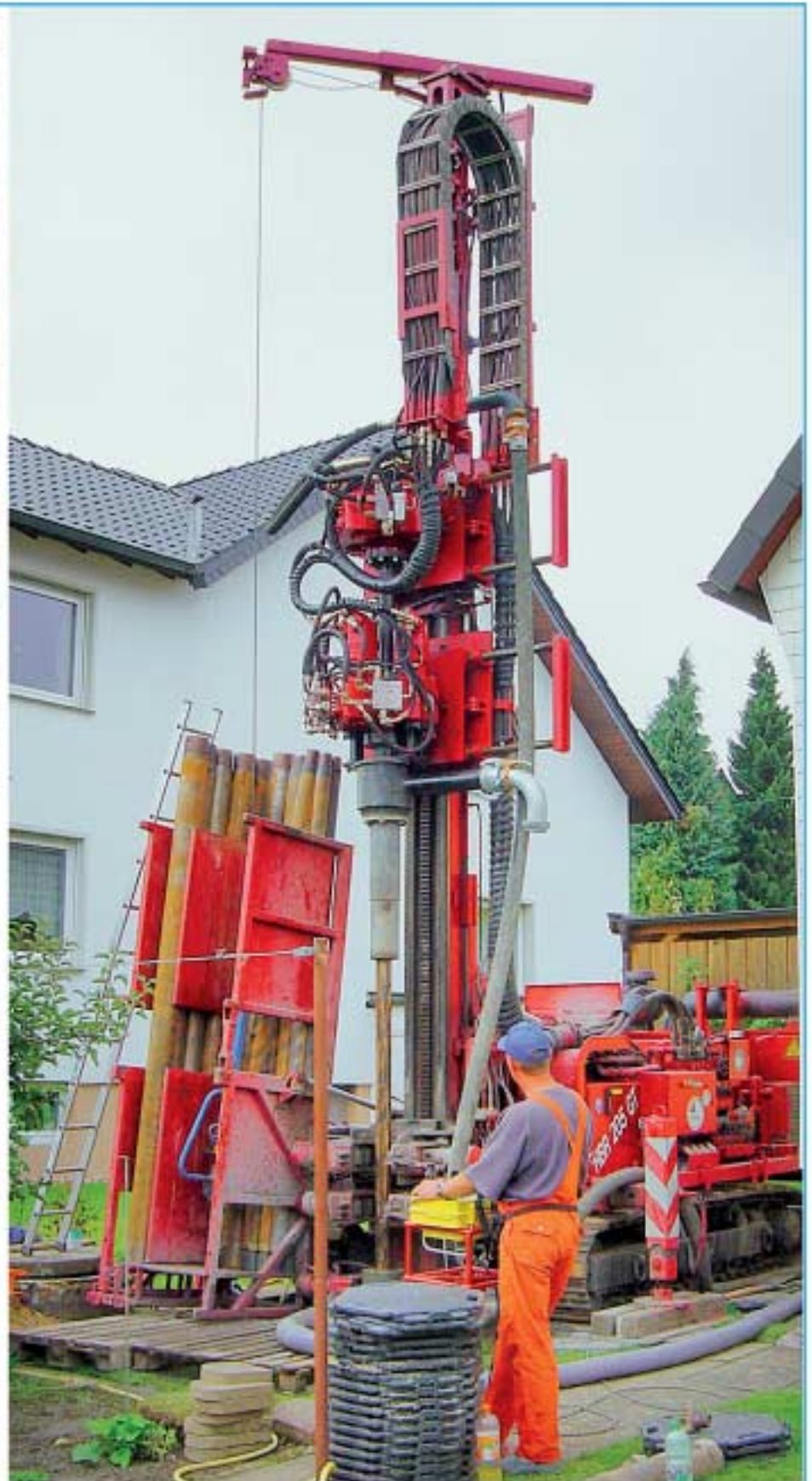
Drill rig type HBR 205 GT with double rotary head type HG24/HG12 equipped with box magazine. Telescopic and swing cat-head.
