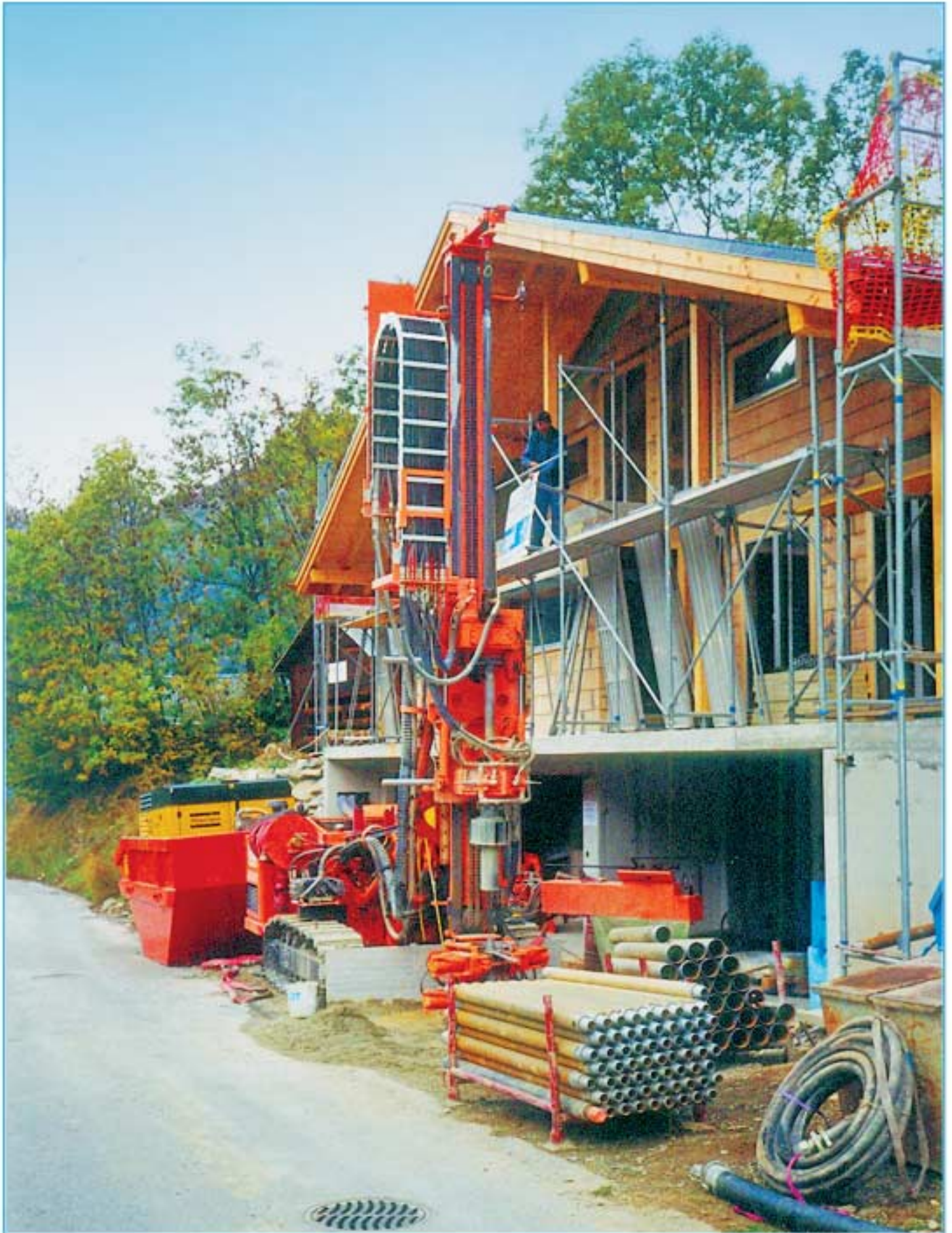
Drill rig type HBR 605, 20 t pull back drill mast for geothermal drilling equipped with double rotary head type HG19/HG11.
