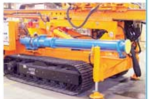
Screw pump for flushing.
